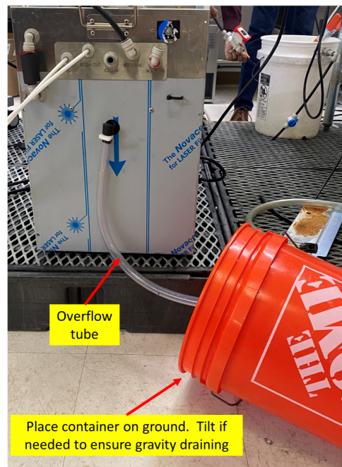
Fill Position: Tube unfastened and pointed down into container
