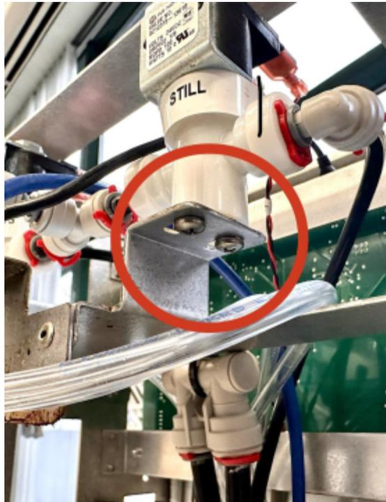
3. Disconnect the tubing from the solenoid
