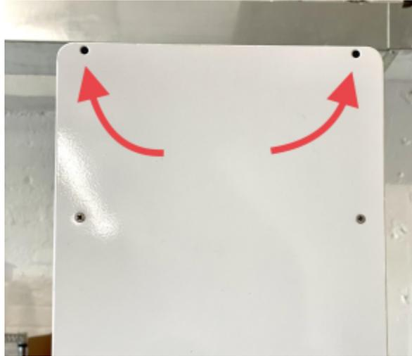
2. Remove the two screws underneath the touchscreen
