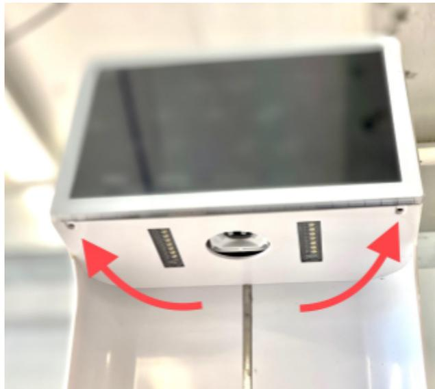
3. Lift the touchscreen and unplug the ethernet, micro USB, and power cables from the touchscreen
