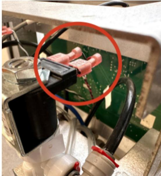
2. Remove the two screws connecting the solenoid to the bracket.
