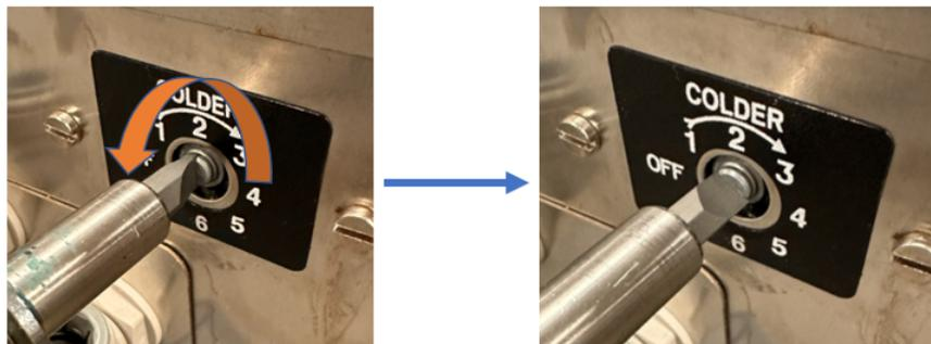
7. With the screwdriver, turn the dial clockwise until you reach the “5” setting. A higher setting is more likely to result in frozen chillers.
