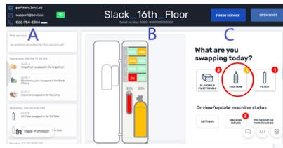
Remember: the indicator shows in Red - meaning "OUT", or Yellow indicating less than 20% remaining.
