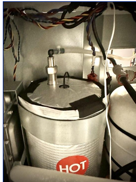
3) Hot water line connection to top of hot water heater/tank
