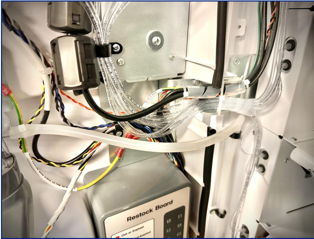
1) Front door assembly with the hot water line connection to the nozzle
