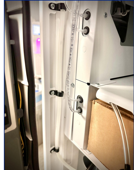
2) Hot water line attachment to the inside of the unit
