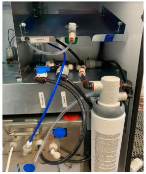
11. Open the valve to the buffer tank.
