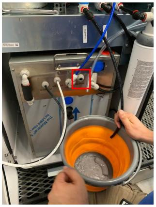
3. After the water tank has been depleted, close the buffer tank valve
