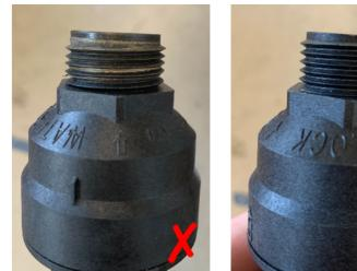
Inspect the tubing on either side of the waterblock fittings. If worn, either replace or cut the current tube to a fresh portion of the tube.
