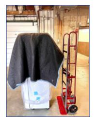
2. Place a moving blanket over the unit to prevent damage.
