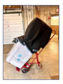
3. One person holds the dolly while the other pushes the unit onto the lower lip and then proceeds to strap the unit to the dolly.
