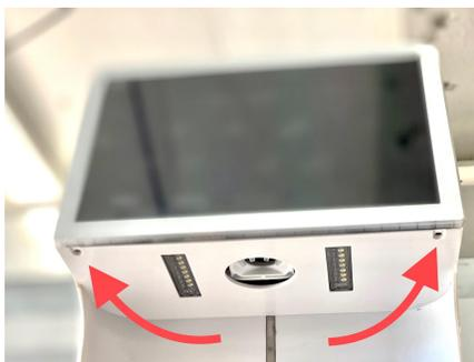
**Note:** Technicians *must* use the furnished hardware from the **Hardware Kit** if swapping from 540-0012 to 540-0042. Furnished #8 x ¼" screws are thread cutting.
