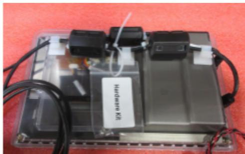
2. Fasten the plastic top cover to the display using the furnished screws and washers.
