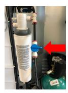
• Position an empty container under the filter flush valve. Open the filter flush valve to **measure the volume of water that exits** the buffer tank through this valve.
