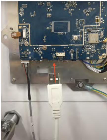
2. Connect the Micro USB end to the control board.
