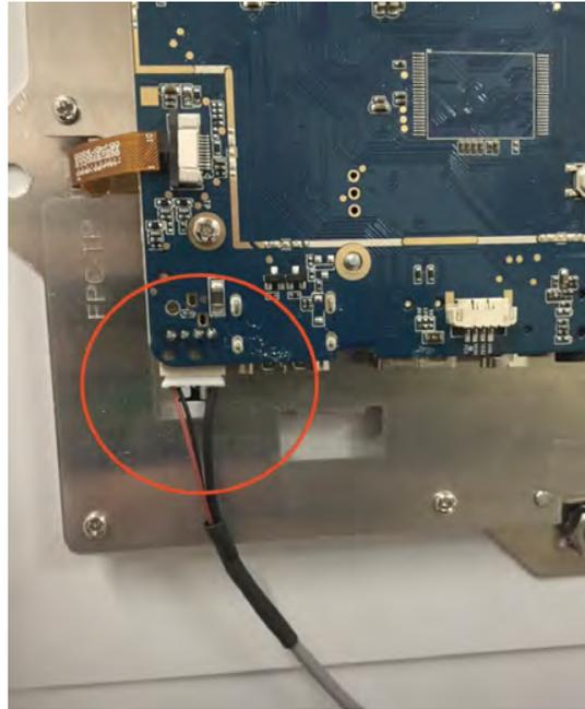
3. Disconnect the LED cable from the control board.
