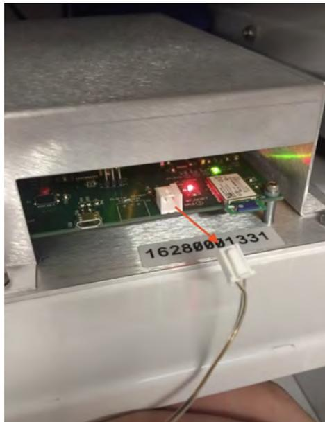
4. Connect the touchscreen power cable to the LED connector on the control board.
