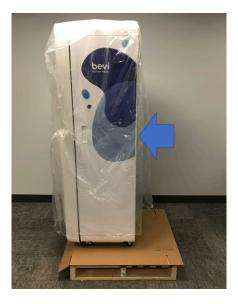
4. Position an appliance cart / hand truck, appropriate for moving this size device, behind the rear of the machine. Use moving blankets / foam supports together with safety straps to secure the machine to the appliance cart. Keep the protective bag in place over the machine whenever moving it.
