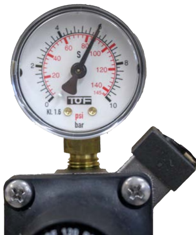
The CO 2 regulator set to a pressure of 6 bar
