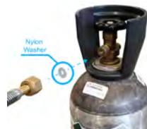
Then, **tighten the hose connector** with an adjustable wrench in a clockwise fashion, following Step 5 but in reverse.
