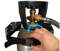
**Shut off the tank** by turning the tank knob **clockwise** until it stops turning.
