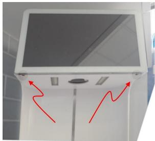
B. Rotate the lid and touchscreen assembly down and forward. Unplug the blue ethernet cable and set the sub-assembly aside.
