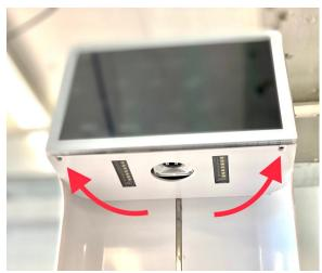
3. Carefully remove the top part of the CT head unit and disconnect the 3 electrical connections (usb, ethernet cable, power)
