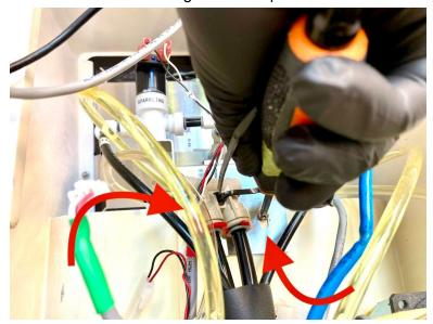
6. Carefully remove the bracket holding the nozzle and solenoids.
