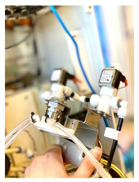
7. Remove the two side screws on the flavor ring and move it out of the way.
