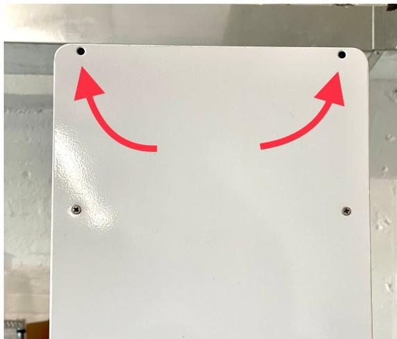
2. Unscrew the 2 screws underneath the front of the head unit.
