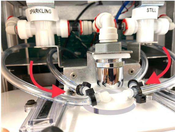
5. Remove and replace aerator using a crescent wrench making sure to place plumber's tape on the threads.
