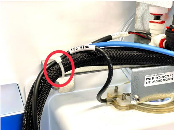
3. Follow the cable bundle and disconnect the LED/Solenoid wire harness.
