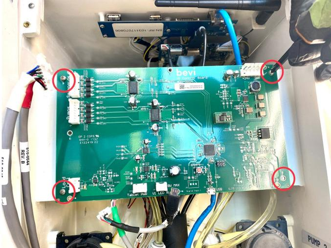
5. Unscrew 2 screws holding bracket in place.
