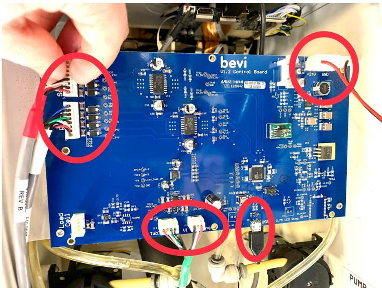
4. Remove the control board by unscrewing the 4 screws in each corner.
