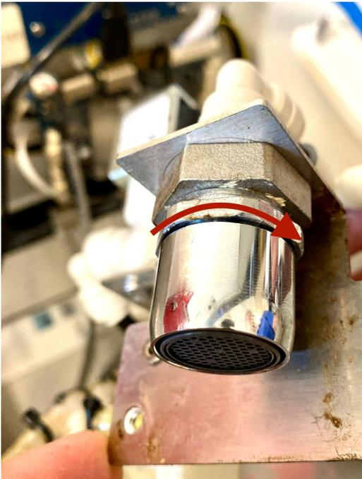
**NOTE: If the upper nut starts to slip during the aerator installation use another crescent wrench to hold it while you tighten the aerator.**
