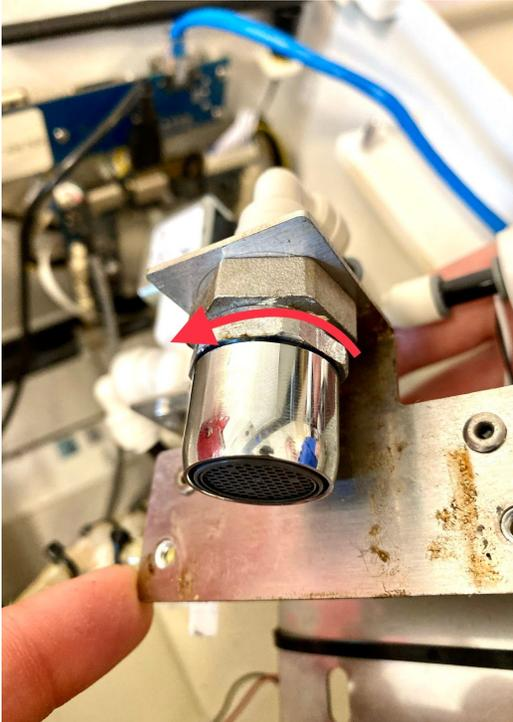
9. Apply plumbers tape on the new aerator threads.
