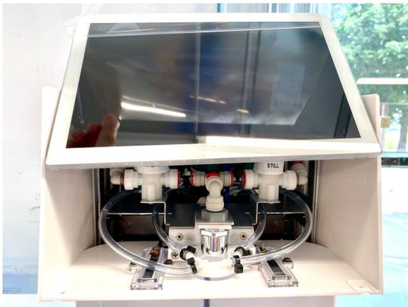
7. Test by holding a container in the dispense area and dispense still and sparkling water. If it is leaking during dispense you may need more plumbers tape or to tighten the aerator further.
