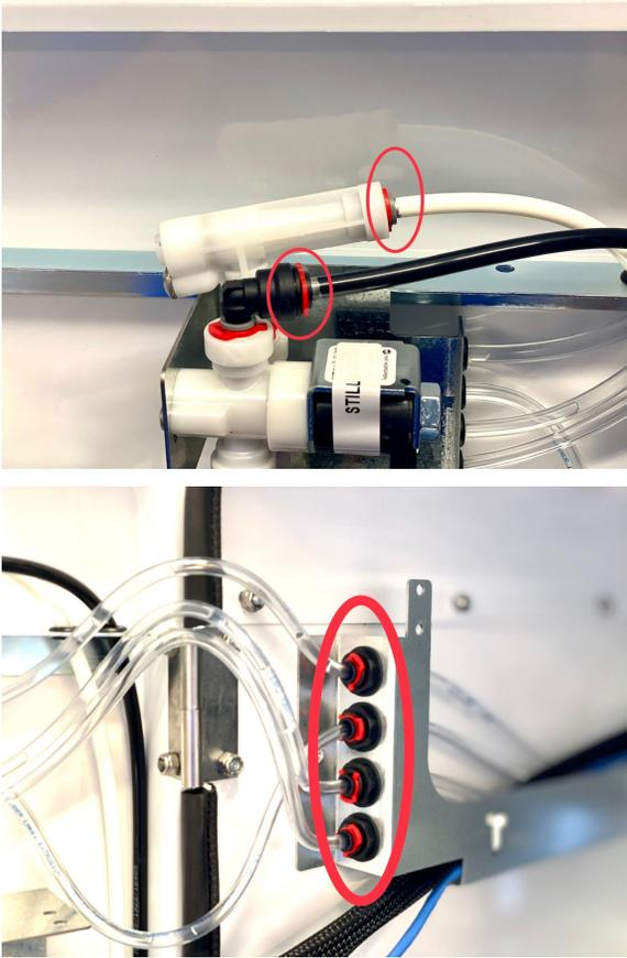
6. Connect the water and flavor tubing to the new assembly performing step 5 in reverse order. Reuse the red clips.
