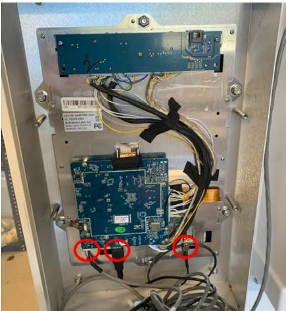
7. Remove the (6) nuts attaching the tablet to the door using a  $\frac{3}{8}$ " socket wrench.
