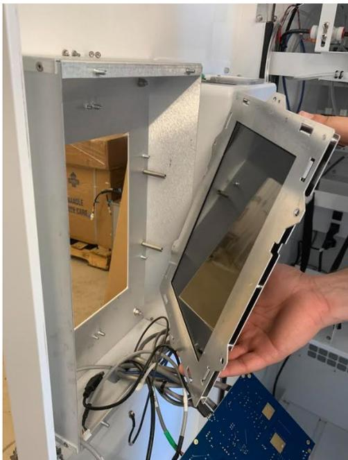
9. To reinstall the tablet assembly, perform steps 3-8 in reverse order.
