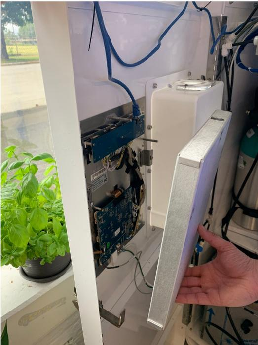
5. Disconnect the following (4) cables: ethernet, power, USB, and grounding wire.
