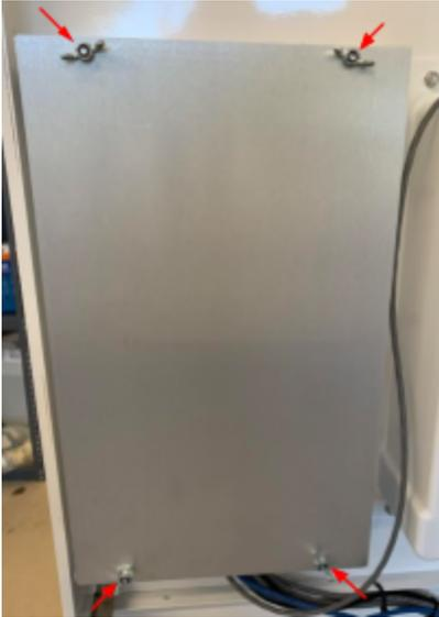
4. Remove the (4) screws from the control board using a #1 phillips screwdriver and disconnect the blue ethernet cable.
