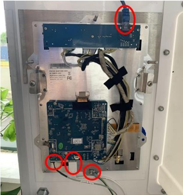
6. Unfasten the (2) screws on either side of the tablet using a #1 Phillips screwdriver.
