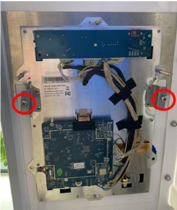
7. Remove the tablet from the studs on the door.
