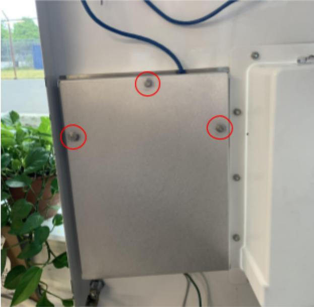
4. Remove the back panel off the studs.
