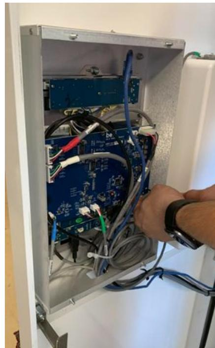
5. Move the control board out of the way so that there is access to the tablet.
