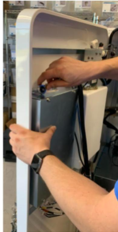
5. Remove the tablet assembly from the door.
