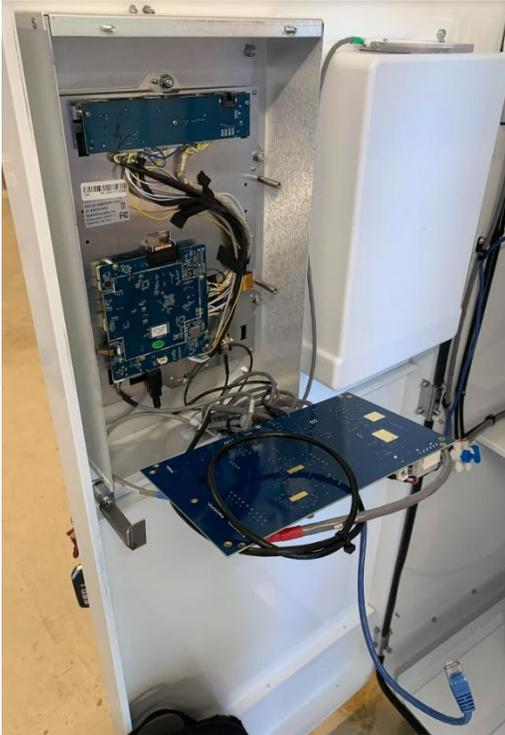
6. Disconnect the following (3) cables: antenna, power, and usb.
