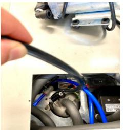
Emptying the Carbonator Tank Without a Pump
