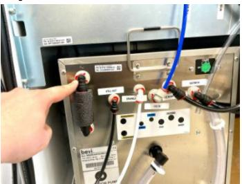
7. Hold a bucket right underneath the fittings and turn the carbonator on. Water should be now pumping into the bucket. Continue until no more water is coming out.
