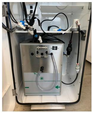
1. Turn off the carbonator by flipping the power switch on the side
