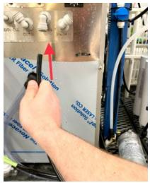
4. Plug the pump into an electrical outlet, and turn on.
