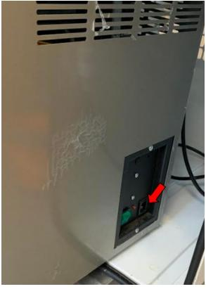
10. Remove the IN WATER and IN CO2 tubes from the back of the unit.
