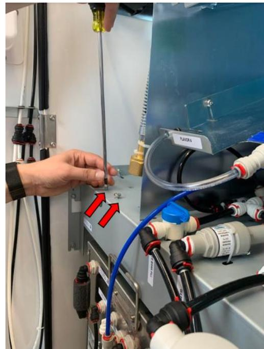
5. Remove the foot clamp and set aside.
