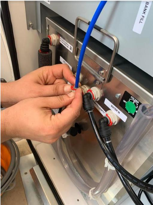
9. Disconnect the tubing that is connected to these (5) fittings.
