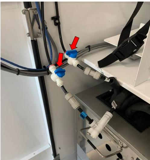
6. Remove the red clips and disconnect the valves, leaving them attached to the carbonator.
