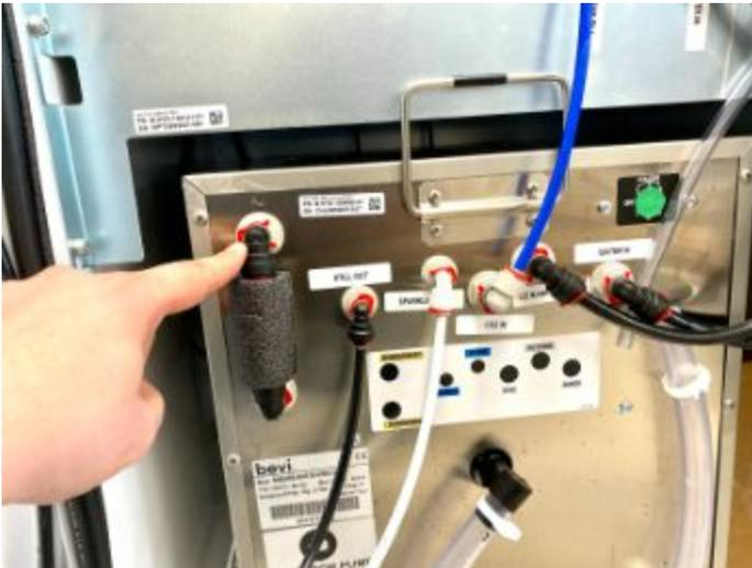
7. Hold a bucket right underneath the fittings and turn the carbonator on. Water should be now pumping into the bucket. Continue until no more water is coming out.
