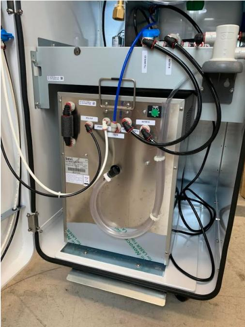
1. Isolate the buffer tank by turning the manual valve to the closed position.
