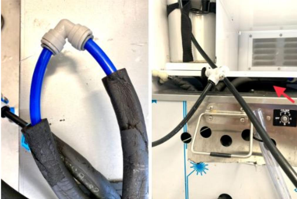
5. Place the two lines coming from the carbonator in the bucket and turn the carbonator on. This will turn on the recirculating pump which will push water out of one of the lines into the bucket. Continue until no more water is coming out.
