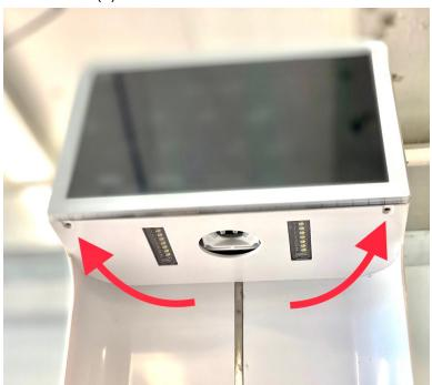
3. Carefully remove the top part of the CT head unit and disconnect the (3) electrical connections (usb, ethernet cable, power)
