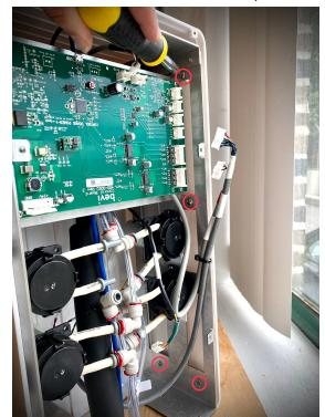
5. Unscrew the touchscreen using the two screws underneath.
