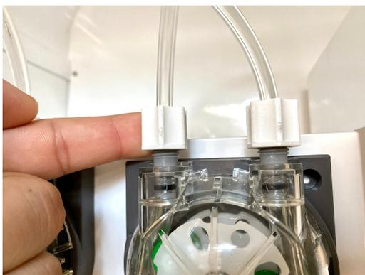
2. Twist off tubing connectors on the pump.
