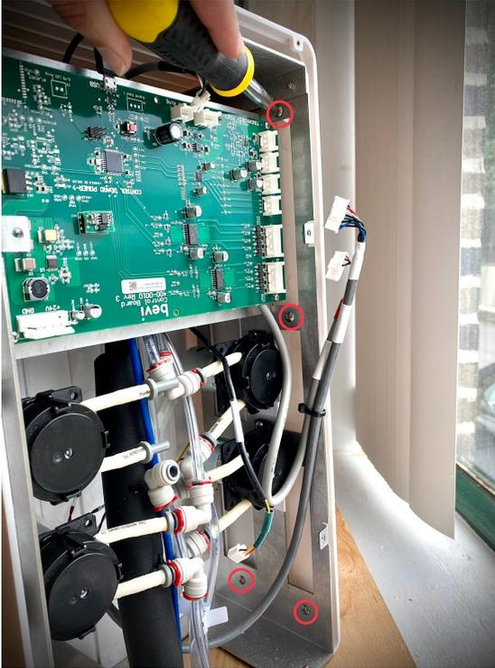
5. Unscrew the touchscreen using the two screws underneath.
