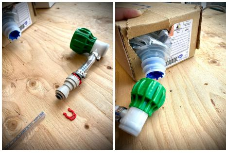
4. Disconnect flavor bib connector (QDC or twist on) from bib.
