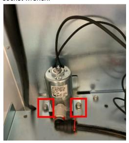
9. Pull the inlet solenoid free from the back panel
