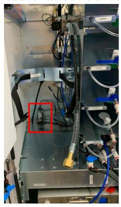
7. Remove the red clip and disconnect the tubing connected to the inlet solenoid.
