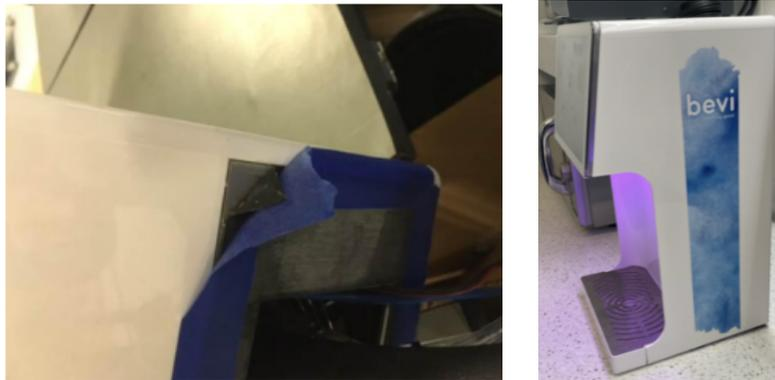
**To resolve:** Simply lift up the console and smooth out the gasket so that there are no wrinkles present. Perform a visual inspection to ensure that the unit is sitting flat on the counter.
