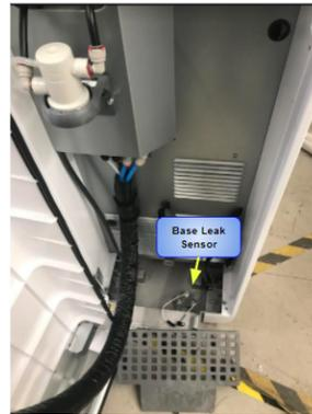
If the sensor is not moving freely - you should replace the sensor.
